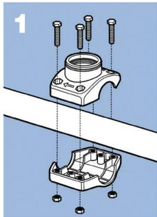
1 Turn pool pump off. Secure clamp assembly on the return line. For above-ground pools with corrugated pipe, use enclosed PVC adapter.
