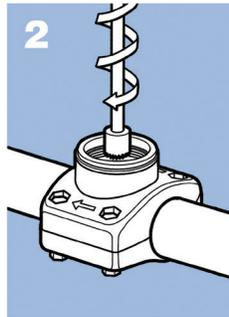
2 Cut hole in rigid PVC pipe using a power drill and the enclosed hole saw.
