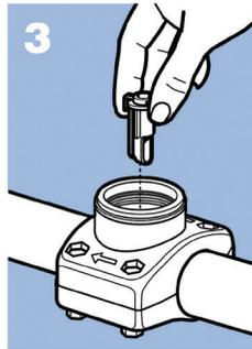
3 Insert the flow diverter into hole and snap it into place.
