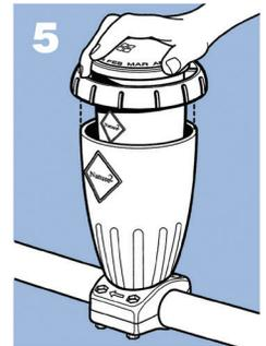
5 Thread the cartridge into the clamp, turn on pool pump and activate the cartridge. See manual for start up instructions.
